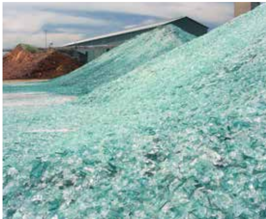
Cullet makes up part of the raw material batch.
